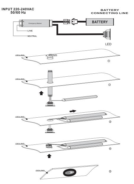
Switch on the power supply and ensure the LED status indicator is illuminated green to ensure the battery and supply are functioning. After 36 hours on continuous charge a mains failure should be simulated to ensure successful operation.
